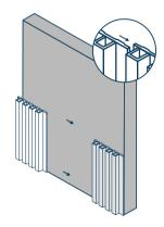
2. Install the second wall panel by placing the long connecting flap over the shorter flap.
