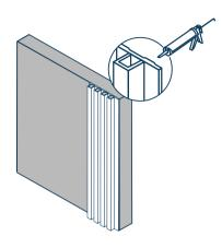
1. Install the first panel, and use construction glue to fix to place
